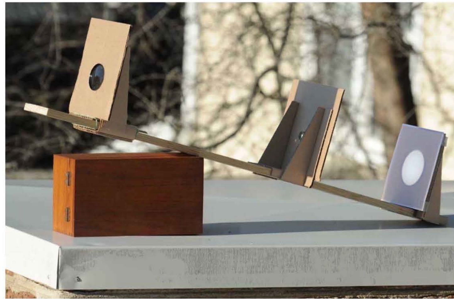
Figure 1. A two-lens Safe Solar Viewer (SSV) as described in this presentation.
