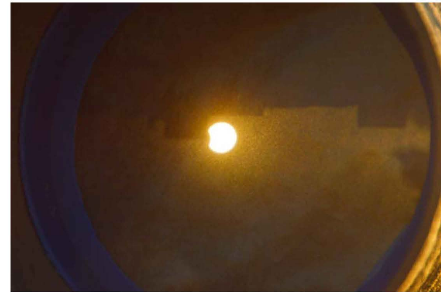
Figure 2. The image made by a 1/2 diopter reading glass viewer on wax paper taped inside the end of a carpet tube.
