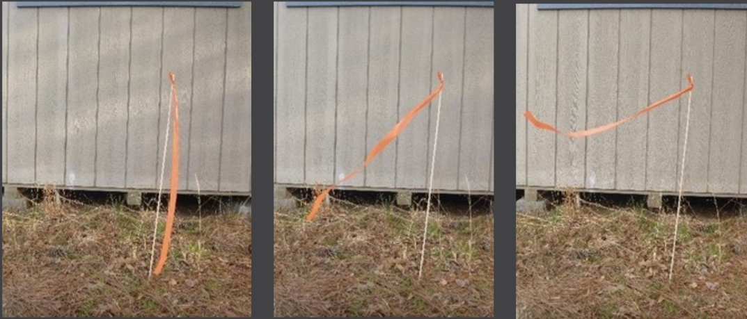
Images of a wind stick showing progressively stronger wind from left to right. Credit: AREN Project
